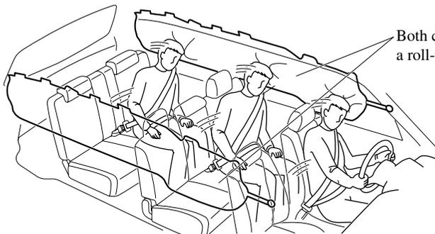
Both curtain air bags will deploy after a roll-over accident is detected.
