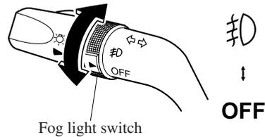
To turn them off, rotate the fog light switch to the OFF position or turn the headlight switch to the
