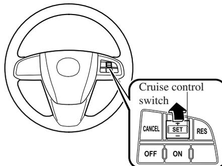
Your vehicle has a tap-up feature that allows you to increase your current speed in increments of 1.6 km/h (1 mph) by a momentary tap of the cruise control SET + switch. Multiple taps will increase your vehicle speed 1.6 km/h (1 mph) for each tap.
