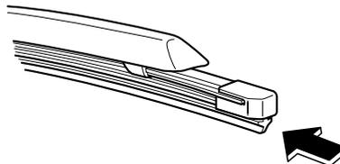
▼ **Replacing Rear Window Wiper Blade**
