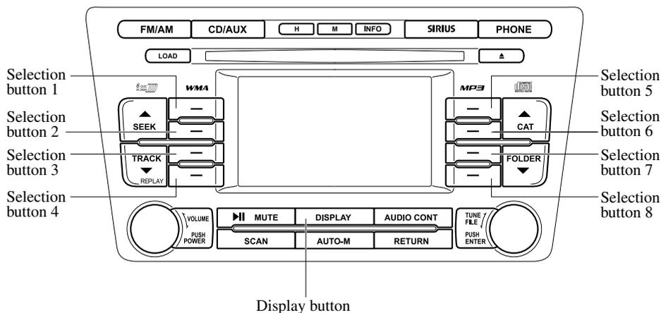
Press the display button ( **DISPLAY** ) to display the tone adjustment screen. Press the button again to return to the previous screen.
