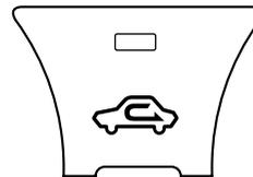
Outside or recirculated air positions can be selected. Press the switch to select outside/recirculated air positions.
