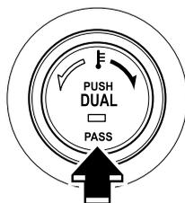
Use the DUAL switch to change the mode between the individual operation (driver and passenger) and interconnection modes.
