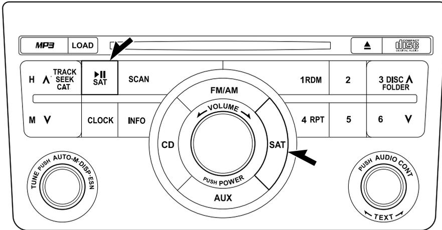
The **▶||** (**SAT**), **SAT** buttons are only functional if the vehicle is equipped with the separately purchased SIRIUS digital satellite radio unit (U.S.A. and Canada).
