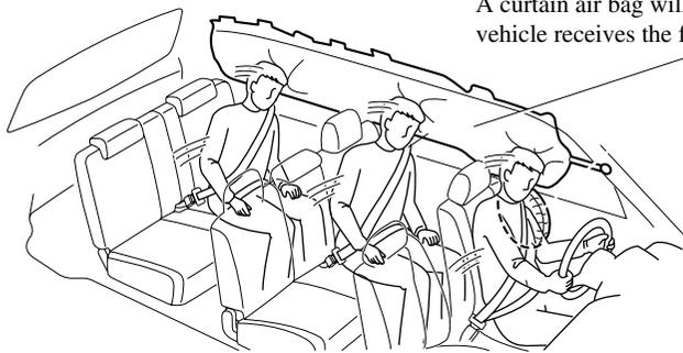
A curtain air bag will deploy only on the side the vehicle receives the force of the impact.
