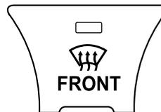
Press the switch to defrost the windshield and front door windows.
