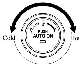
This dial controls temperature. Turn it clockwise for hot and counterclockwise for cold.
