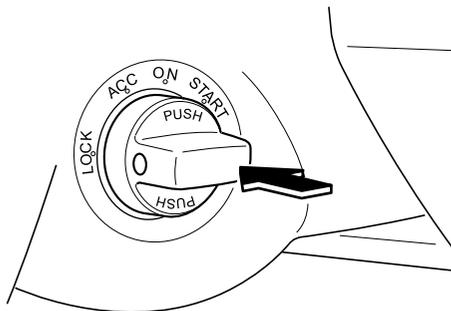
7. Verify that the KEY indicator light (green) illuminates in the instrument cluster. The KEY warning light (red) means you cannot continue to start the engine using the Advanced Keyless System. You may have to use the auxiliary key instead (page 3-22).
