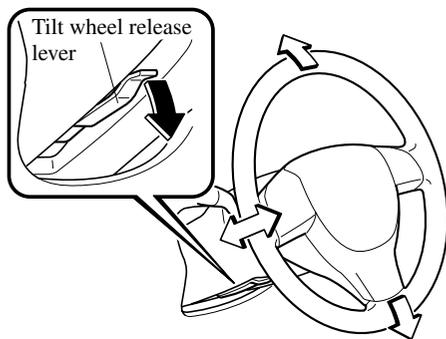
2. Tilt the steering wheel and/or adjust the steering column length to the desired positions, push the lever up to lock the column.
