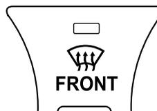
Press the windshield defroster switch. In this position, the
