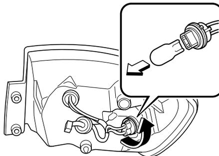
4. Disconnect the bulb from the socket.
