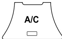
Pressing the A/C switch while the AUTO switch is turned on will turn off the air conditioning (cooling/dehumidifying functions). The air conditioning can be turned on and off by pressing the A/C switch while the fan control dial is on.
