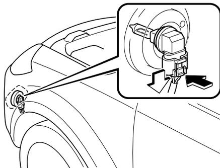
5. Turn the socket and bulb assembly counterclockwise and remove it. Carefully remove the bulb from its socket in the reflector by gently pulling it straight backward out of the socket.
