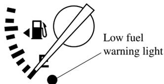
This warning light in the fuel gauge signals that the fuel tank will soon be empty. Refuel as soon as possible.
