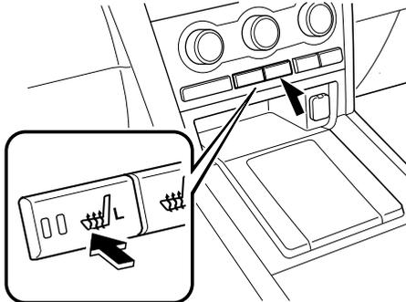
Press the seat warmer switch to illuminate the indicator light while the ignition switch is turned to the ON position. The mode changes as follow each time the seat warmer switch is pressed.
