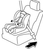
**Seating a child in a child-restraint system on the front passenger seat is dangerous (With Driver and Front Passenger Occupant Classification System):**
