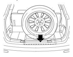
11. Thread the belt through the wheel as shown in the figure, then attach the belt clips to the attachment loop.
