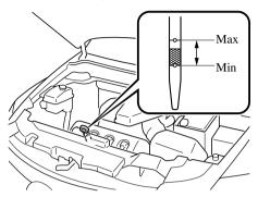
5. Pull it out again and examine the level. The level is normal if it is between MIN and MAX. If it is below MIN, add oil to raise the level within the hatching zone.
