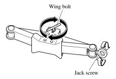
3. Turn the wing bolt completely to secure the jack.
