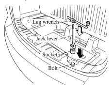
Slowly turn the lug wrench counterclockwise until the spare tire reaches the ground and the cable becomes loose.
