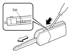
3. Insert a screwdriver into the slot and gently pry open the transmitter.
