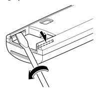
3. Insert the small, flathead screwdriver into the gap between the cover and the transmitter, and then rotate the screwdriver to detach the cover.
