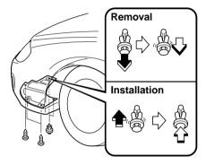
Disconnect the electrical connector from the bulb by pressing the tab on the connector with your finger and pulling the connector downward.
