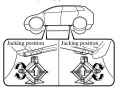
Continue raising the jack head gradually by rotating the screw with your hand until the jack head is inserted into the jack-up position.
