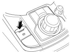
If the EPB switch is pressed without depressing the brake pedal, the display or indicator light in the instrument cluster notifies the driver that the brake is not depressed.
