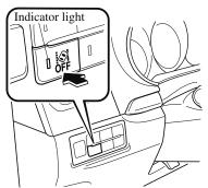
Drive the vehicle in the center of the driving lane while the LAS&LDWS OFF switch indicator light is turned off. The system becomes operational when all of the following conditions are met.
