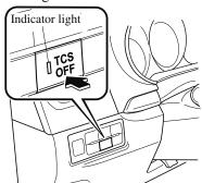
Press the switch again to turn the TCS back on. The TCS OFF indicator light and TCS OFF switch indicator light will turn off.
