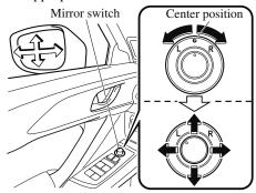
After adjusting the mirror, lock the control by rotating the switch in the center position.
