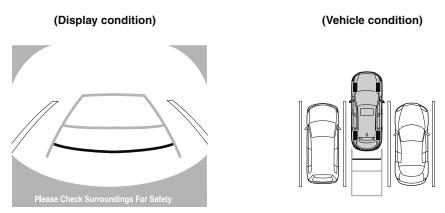
6. When the selector lever is shifted from reverse (R) to another selector lever position, the screen returns to the previous display.
