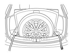
4. Pass the flat tire belts through the wheel of the flat tire.
