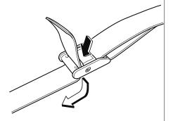
2. Hook the clips of the flat tire belts to the hooks under the third-row seat.
