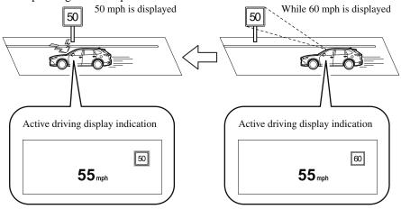
The excessive speed warning is initially set to inoperable. If you want to activate the excessive speed warning, change the setting in the personalization features. In addition, the warning pattern and the warning activation timing differ depending on the setting contents. Refer to Personalization Features on page 9-11.
