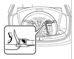
6. While pressing the flat tire against the third-row seat, pull the ends of the flat tire belts and secure the flat tire.
