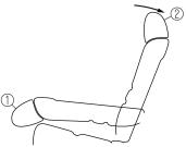
2. Make sure the seatback is securely latched by pushing it back until it is fully locked.
