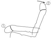
3. Make sure the seatback is securely latched by pushing it back until it is fully locked.
