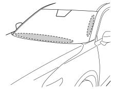
The windshield wiper de-icer operates in conjunction with the rear window defogger.
