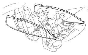
Both curtain air bags will deploy after the roll-over accident is detected.
