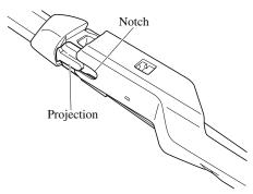
10. Slide the blade component and install it to the wiper arm.
