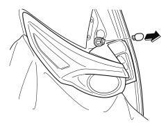
9. Install the new bulb in the reverse order of the removal procedure.
