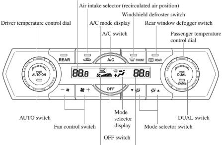
Airflow display Temperature setting display (Passenger's side)
