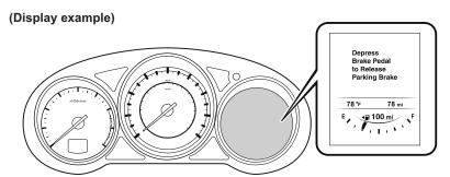
If the warning light turns on/flashes simultaneously or a symbol is indicated in the display, check the information regarding the warning light or symbol. (page 4-31)
