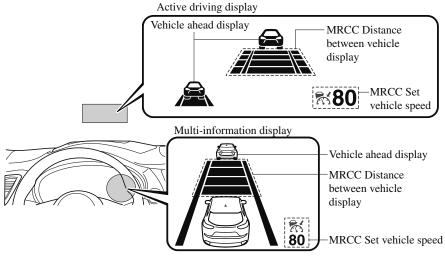
If there is a problem with the MRCC with Stop & Go function system, a message is displayed on the multi-information display. Check the center display to verify the problem and then have your vehicle inspected by an Authorized Mazda Dealer. Refer to Message Indicated on Display on page 7-44.
