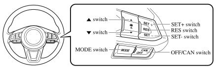
When the MODE switch is pressed once, the MRCC with Stop & Go function system turns on, and the MRCC with Stop & Go function main indication (white) turns on and the vehicle speed and the distance between the vehicles while in headway control can be set.
