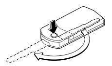
To retract the key, rotate it into the holder while pressing the release button.
