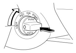
Turn the ignition switch from the ACC position to the START position and hold (up to 10 seconds at a time) until the engine starts.
