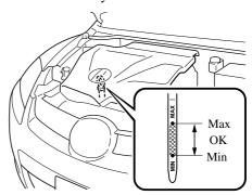
6. Pull it out again and examine the level. It's OK between MIN and MAX. But if it's near or below MIN, add enough oil to bring the level to MAX.
