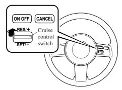
Your vehicle has a tap-up feature that allows you to increase your current speed in increments of 1.6 km/h (1 mph) by a momentary tap of the cruise control RES/+ switch. Multiple taps will increase your vehicle speed 1.6 km/h (1 mph) for each tap.
