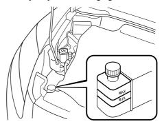
The level must be kept between MAX and MIN.
