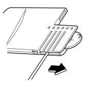
4. Insert the new battery (CR2025 or equivalent) with the positive pole (+) facing the (+) mark on the cap.
