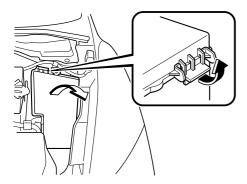
Pull the fuse straight out with the fuse puller provided on the inside of the engine compartment fuse block cover.
