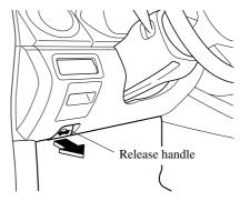
Insert your hand into the hood opening and Slide the hood latch to the right and lift the hood.
