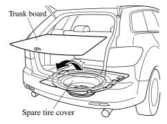
2. Turn the tire hold-down bolt counterclockwise with the lug wrench.
