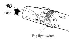
To turn them off, rotate the fog light switch to the OFF position or turn the headlight switch to the ● or OFF position.
