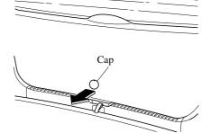
2. Turn the lever to the right to unlock the liftgate.
