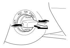
4. Insert the auxiliary key in the ignition switch.
