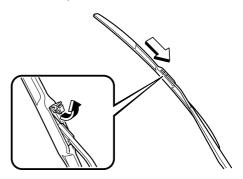
3. Tilt the blade assembly and remove it from the arm.
