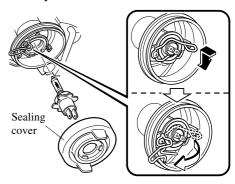
8. Carefully remove the bulb from the socket by pulling it straight back.
