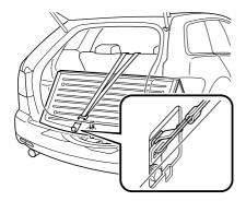
5. Push the trunk board down to its original position.
