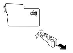
4. If any fuse but the MAIN fuse is blown, replace it with a new one of the same amperage rating.
