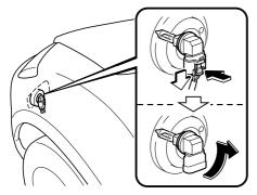
6. Install the new bulb in the reverse order of removal.
