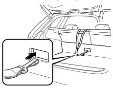
3. Latch the hook onto the anchor bracket
