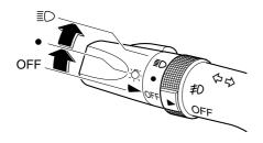
Turn the headlight switch to turn the headlights, other exterior lights and dashboard illumination on or off.
