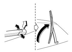
2. Firmly rotate the wiper blade to the right until it unlocks, then remove the blade.
