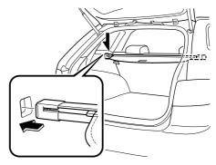
2. Squeeze the spring holder on right end of the retractor bar inward, then insert it into the notch.
