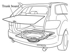
Turn the wing bolt and jack screw counterclockwise.
