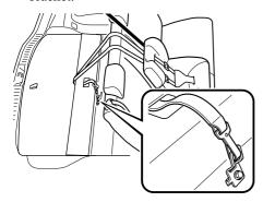
4. Push the trunk board down to its original position, and tighten the tether strap following the child-restraint system manufacturer's instructions.
