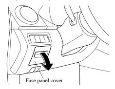
Pull the fuse straight out with the fuse puller provided on the inside of the cover for the fuse panel and the fuse block cover inside of the engine compartment.
