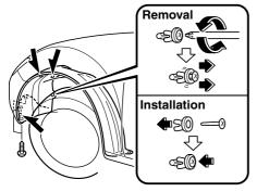
4. Detach the electrical connector from the bulb by pulling it to the rear.
