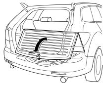
4. Latch the hook onto the anchor bracket, and tighten the tether strap following the child-restraint system manufacturer's instructions.
