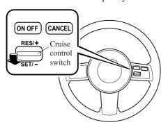
Your vehicle has a tap-down feature that allows you to decrease your current speed in decrements of 1.6 km/h (1 mph) by a momentary tap of the cruise control SET/switch. Multiple taps will decrease your vehicle speed 1.6 km/h (1 mph) for each tap.
