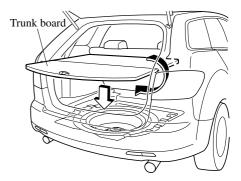
3. Fold the trunk board into the position shown in the figure.
