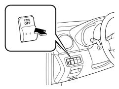
Press the switch again to turn the TCS back on. The TCS OFF indicator light will go out. If the vehicle speed is more than 30 km/h (18 mph), the TCS OFF indicator light will not illuminate even if the switch is pressed.
