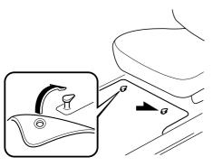
When setting a floor mat, position the floor mat so that its eyelets and inserted over the pointed end of the retention posts.
