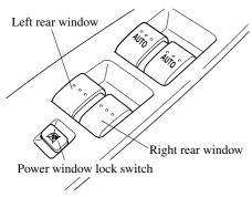
To open the power window to the desired position, hold down the switch.
