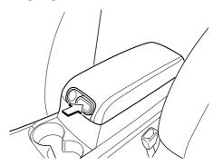
The center console has a lockable lid, insert the key into the slot; then turn the key clockwise to lock, counterclockwise to unlock.
