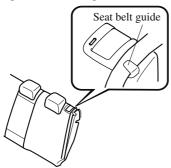
Press the seatback rearward and lock it in place. After returning the seatback to its upright position, make sure it is securely locked.
