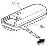
4. Twist the flathead screwdriver in the direction of the arrow and remove the cover.
