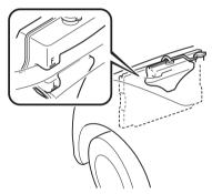
If it is at or near L, add enough coolant to the coolant reservoir to provide freezing and corrosion protection and to bring the level to F.
