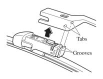
9. Align the blade component projection with the wiper arm notch.
