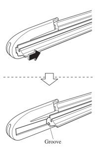
4. Pull the end of the blade rubber from the blade holder groove in the direction of the arrow and remove the blade rubber from the blade holder.
