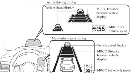
If there is a problem with the Mazda Radar Cruise Control with Stop & Go function (MRCC with Stop & Go function) system, a message is displayed on the multi-information display. Check the center display to verify the problem and then have your vehicle inspected by an Authorized Mazda Dealer.
