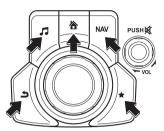
The following operations can be done by pressing the switches around the commander knob.
