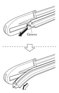
5. Insert the end of the new blade rubber into the groove of the blade holder until it contacts the end of the blade holder.
