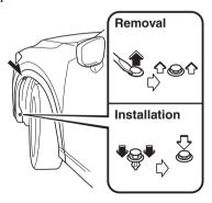
4. Pull the center of each plastic retainer using a flathead screwdriver and remove the retainers, and then partially peel back the mudguard.
