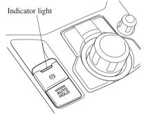
Firmly depress the brake pedal and press the electric parking brake (EPB) switch. If the electric parking brake (EPB) switch is pressed without depressing the brake pedal, the display or indicator light in the instrument cluster notifies the driver that the brake is not depressed.
