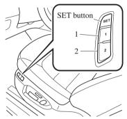
The driving position can be programmed or operated using the buttons on the side of the seat or the key.
