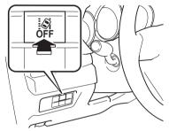
The Lane-keep Assist System (LAS) & Lane Departure Warning System (LDWS) OFF indicator light turns on.
