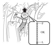
The top of the float should be between F and L.
