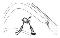
Disconnect the electrical connector from the bulb by pressing the tab on the connector with your finger and pulling the connector.
