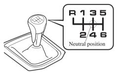
The shift pattern of the transaxle is conventional, as shown.
