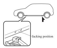
6. Continue raising the jack head gradually by rotating the screw with your hand until the jack head is inserted into the jack-up position.
