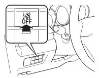
Drive the vehicle in the center of the driving lane while the Lane-keep Assist System (LAS) & Lane Departure Warning System (LDWS) OFF indicator light in the instrument cluster is turned off.
