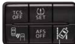
Use the LDWS switch to turn system ON or OFF
