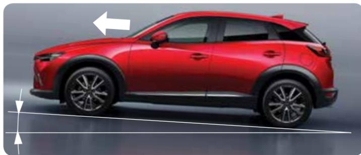
When the brake pedal is released and the accelerator pedal is pushed, HLA prevents the vehicle from rolling forward or backward. It operates on a downward slope when the shift lever is in the reverse (R) position, and on an upward slope when the shift lever is in a position other than the reverse (R) position.
