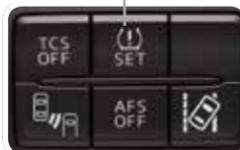
**CAUTION:** If the TPMS “Set Switch” is pushed without adjusting the tire pressure, the system cannot detect the normal tire pressure. The TPMS warning light may not turn on, even if the tire pressure is low, or it may turn on if the tire pressure is normal.
