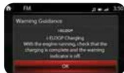
When this warning screen appears, do not drive the vehicle. Allow the engine to idle until the warning screen disappears. This time is needed for normal generator operation.
