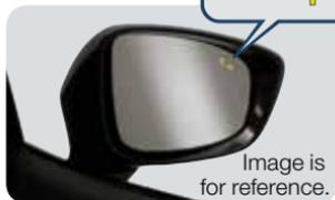
**WARNING:** RCTA is only a supplementary system to help aid when backing up, however RCTA has limitations. The system does not detect all vehicles, especially a motorcycle. Do not rely solely on the RCTA. Relying solely on the RCTA may cause an unexpected accident resulting in serious injury. Always back up slowly.
