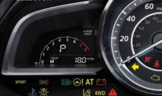
**IMPORTANT:** When your Mazda Connect display setting is set on "AUTO", the instrument cluster and display may become dimmer when the headlights are on. If the display and instrument cluster become too dim or too bright when the headlights are on, simply rotate the dimmer knob located on your instrument cluster to adjust the brightness.
