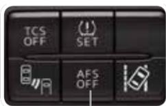
Push AFS OFF to turn system off or on. When off, the AFS OFF indicator in the instrument panel will turn on.
