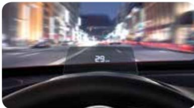
**CAUTION:** Always adjust the display using the Settings screen (AD-Disp tab). Do not try to adjust the angle or open/close the display by hand. Fingerprints on the display will make it difficult to view and manual operation could cause damage.
