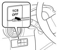
Press the switch again to turn the TCS back on. The TCS OFF indicator light will turn off.
