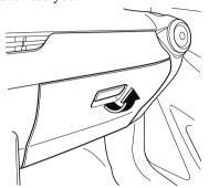
To close the glove compartment, firmly press in the center of the glove compartment lid.
