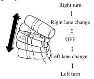
The turn signal indicators in the instrument cluster flash according to the operation of the turn signal lever to show which signal is working.
