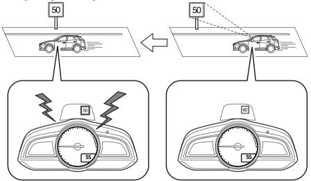
The excessive speed warning is initially set to inoperable. If you want to activate the excessive speed warning, change the setting in the personalization features. In addition, the warning pattern and the warning activation timing differ depending on the setting contents. Refer to Personalization Features on page 9-9.
