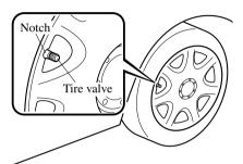
Damage could occur during installation if the wheel cover is not properly aligned.
