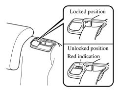
1. Make sure that the seat belt passes through the seat belt guide correctly and it is not twisted, then raise the seatback while preventing the seat belt from being caught in the seatback.
