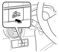
Press the switch again to turn the system back on. The Smart City Brake Support (SCBS) OFF indicator light will turn off.
