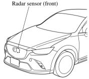
If the Smart Brake Support/Smart City Brake Support (SBS/SCBS) Warning Light (amber) is illuminated, the area around the radar sensor may be dirty. Refer to "Warning Guidance" in the center display (Type B audio).
