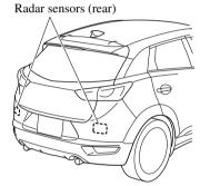
The radar sensors (rear) are installed inside the rear bumper, one each on the left and right sides.
