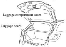
Lower the liftgate slowly using the liftgate grip recess, then push the liftgate closed using both hands.
