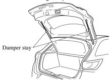
➤ Do not modify or replace the liftgate damper stay. Consult an Authorized Mazda Dealer if a liftgate damper stay is deformed or damaged for reasons such as a collision or if there is some other problem.
