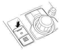
If the EPB switch is pressed without depressing the brake pedal, the indicator light in the instrument cluster notifies the driver that the brake is not depressed. The brake pedal operation demand indicator light (green) in the instrument cluster turns on.
