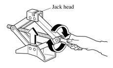
Place the jack under the jack-up position closest to the tire being changed with the jack head squarely under the jack-up point.
