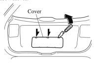
3. Using a flathead screwdriver, open the inner cover.
