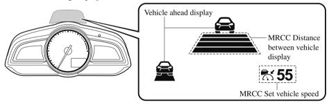
If there is a problem with the MRCC with Stop & Go function system, MRCC with Stop & Go function warning light (amber) turns on. Check the center display to verify the problem and then have your vehicle inspected by an Authorized Mazda Dealer.
