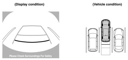
6. When the shift lever/selector lever is shifted from R to another shift lever/selector lever position, the screen returns to the previous display.
