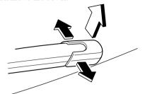
2. Remove the stopper and raise the wiper arm.
