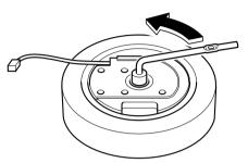
For vehicles not equipped with a sub-woofer, turn the spare tire hold-down bolt counterclockwise and remove the spare tire.
