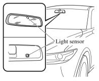
• The auto-dimming function is canceled when the ignition is switched ON and the selector lever is in reverse (R).
