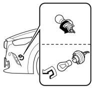
5. Install the new bulb in the reverse order of the removal procedure.
