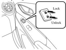
To lock all the doors and the liftgate from an open front door, press the lock side of the door lock switch and then close the door.
