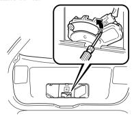
4. Using a flathead screwdriver, turn the lever to the right to unlock the liftgate.
