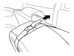
15. Insert the luggage compartment cover from the top of the luggage compartment opening with the cloth side of the cover facing outward, and slide it between the flat tire and the inside perimeter of the luggage compartment opening.
