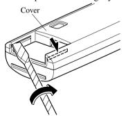
3. Insert the tape-wrapped flathead screwdriver into the gap and slide it in the direction of the arrow.
