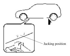
Continue raising the jack head gradually by rotating the screw with your hand until the jack head is inserted into the jack-up position.
