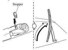
3. Firmly rotate the wiper blade to the right until it unlocks, then remove the blade.
