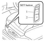
A driving position can be programmed or operated using the buttons on the side of the seat or the key.
