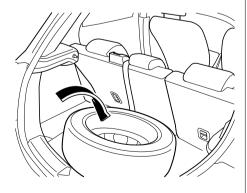
12. Thread the buckle through the wheel as shown in the figure.
