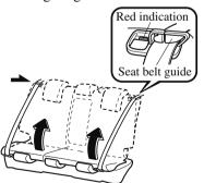
2. Press the seatback rearward and lock it in place. After returning the seatback to its upright position, make sure it is securely locked.
