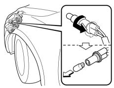
4. Install the new bulb in the reverse order of the removal procedure.
