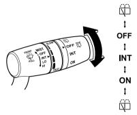
Turn the wiper on by turning the rear wiper/washer switch.
