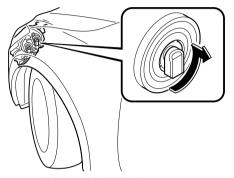
5. Install the new bulb in the reverse order of the removal procedure.
