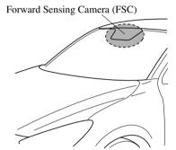
The Forward Sensing Camera (FSC) determines the conditions ahead of the vehicle while traveling at night and detects traffic lanes. The distance in which the Forward Sensing Camera (FSC) can detect objects varies depending on the surrounding conditions.
