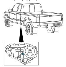
3. Add only enough fluid through the filler opening so that the fluid level is at the bottom of the opening.
