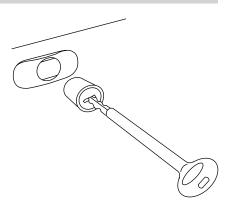
3. Insert the straight end of the jack handle into the rear access hole located just above the rear bumper and below the tailgate.
