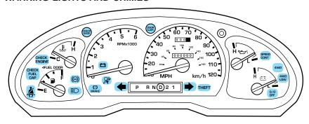
Warning lights and gauges can alert you to a vehicle condition that may become serious enough to cause expensive repairs. A warning light may illuminate when a problem exists with one of your vehicle's functions. Many lights will illuminate when you start your vehicle to make sure the bulb works. If any light remains on after starting the vehicle, have the respective system inspected immediately.
