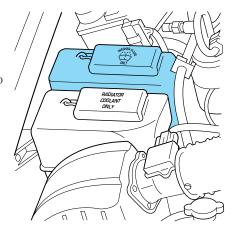
Only use a washer fluid that meets Mazda specification . Refer to  $Lubricant\ specifications$  in this chapter.
