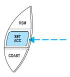
**NOTE:** You can accelerate with the accelerator pedal at any time during speed control usage. Releasing the accelerator pedal will return your vehicle to the previously programmed set speed.
