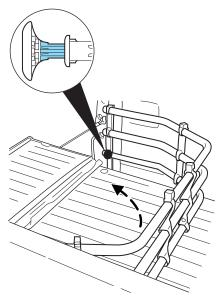
4. Evenly push down on the extender and push the round knobs in on each side locking it in place.
