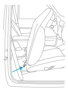
3. Locate the correct anchor for the selected seating position.
