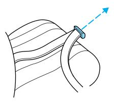
Shorten and fasten the belt when not in use to keep the belt away from door openings and available after unfolding the seats.
