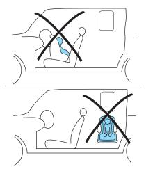
WARNING: Rear facing child seats should NEVER be placed in the front seats unless the passenger airbag switch is turned off. See *Passenger airbag ON/OFF switch* in this chapter.
