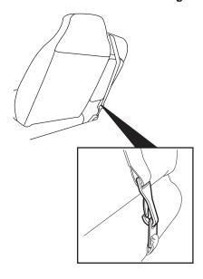
When installing a child safety seat in the center position, route the tether strap over the center arm rest and clip it to the center anchor.
