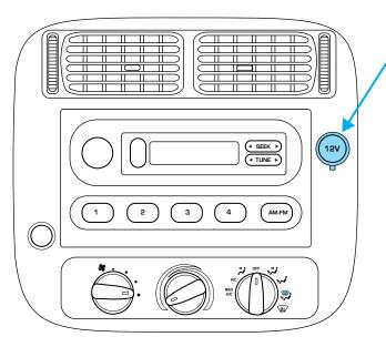
Power outlets are designed for accessory plugs only. Do not hang any type of accessory or accessory bracket from the plug. Improper use of the power outlet can cause damage not covered by your warranty.
