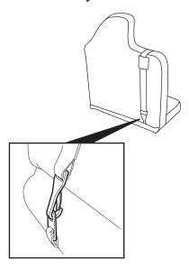
When installing a child safety seat in the center position on a 60/40 vinyl seat, route the tether strap through the guiding sleeve and clip it to the center anchor.
