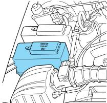
When the engine is cold, check the level of the engine coolant in the reservoir.
