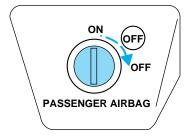
WARNING: If the OFF light fails to illuminate when the passenger air bag switch is in the OFF position and the ignition switch is in ON, have the passenger air bag switch serviced at you authorized Mazda dealership.
