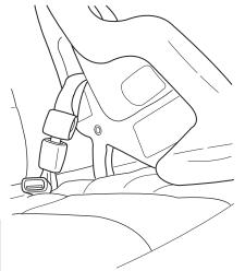
• Keep the buckle release button pointing up and away from the safety seat, with the tongue between the child seat and the release button, to prevent accidental unbuckling.
