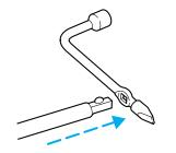
2. If equipped, unlock and remove the spare tire carrier lock from the rear access hole located just above the rear bumper and below the tailgate.
