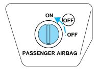
WARNING: If the light is illuminated when the passenger air bag ON/OFF switch is in the ON position and the ignition switch is ON, have the passenger air bag ON/OFF switch serviced at your authorized Mazda dealership immediately.
