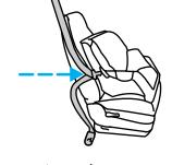
4. Insert the belt tongue into the proper buckle (the buckle closest to the direction the tongue is coming from) for that seating position until you hear and feel the latch engage. Make sure the tongue is latched securely by pulling on it.
