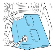
However, for severe usage or in high temperature climates, check the battery electrolyte level. Refer to the service maintenance section for the service interval schedules.
