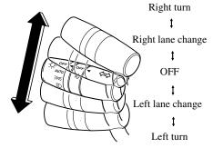
The turn signal indicators in the instrument cluster flash according to the operation of the turn signal lever to show which signal is working.
