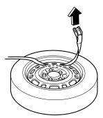
13. Pass the belt through the buckle, then pull the belt end to secure the flat tire.
