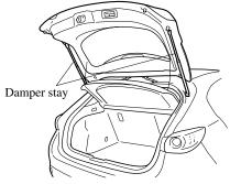
Do not modify or replace the liftgate damper stay. Consult an Authorized Mazda Dealer if a liftgate damper stay is deformed or damaged for reasons such as a collision or if there is some other problem.
