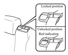
1. Make sure that the seat belt passes through the seat belt guide correctly and it is not twisted, then raise the seatback while preventing the seat belt from being caught in the seatback.
