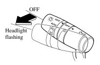
The headlight high-beam indicator light in the instrument cluster illuminates simultaneously. The lever will return to the normal position when released.
