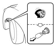
Parking lights/Front side-marker lights (With halogen headlights), Front side-marker lights (With LED headlights)
