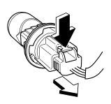
Disconnect the bulb by pulling it out.
