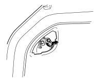
4. Disconnect the connector from the unit by pressing the tab on the connector with your finger and pulling the connector.
