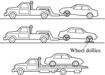
When towing with the rear wheels on the ground, release the parking brake. Refer to Parking Brake on page 4-61. Refer to Electric Parking Brake (EPB) on page 4-61.
