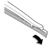
5. Remove the metal stiffeners from the blade rubber and install them in the new blade.
