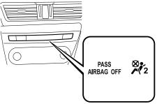
If the front passenger occupant classification sensor is normal, the indicator light turns on when the ignition is switched ON. The light turns off after a few seconds. Then, the indicator light turns on or is off under the following conditions:
