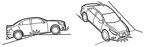
This vehicle is equipped with low profile tires allowing class-leading performance and handling. As a result, the sidewall of the tires are very thin and the tires and wheels can be damaged if driven through potholes or on rough/uneven roads at excessive speeds. Use care and reduce speed when traveling on rough/uneven roads or through potholes.
