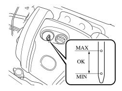
Pull it out again and examine the level. The level is normal if it is between the MIN and MAX marks.
