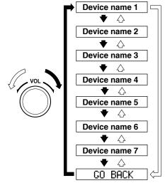
Press the audio control dial to select the device you would like to link. The
