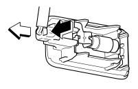
3. Disconnect the bulb by pulling it out.
