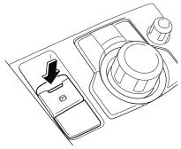
If the EPB switch is pressed without depressing the brake pedal, the indicator light in the instrument cluster notifies the driver that the brake is not depressed. The brake pedal operation demand indicator light in the instrument cluster turns on.
