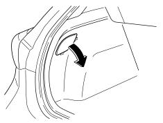
Turn the socket and bulb assembly counterclockwise and remove it.
