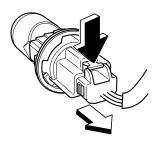
8. Disconnect the bulb by pulling it out. Rear turn signal lights, Brake lights/ Taillights/Rear side-marker lights (Bulb type)
