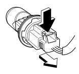
7. Disconnect the bulb by pulling it out. Rear turn signal lights, Brake lights/ Taillights/Rear side-marker lights (Bulb type)
