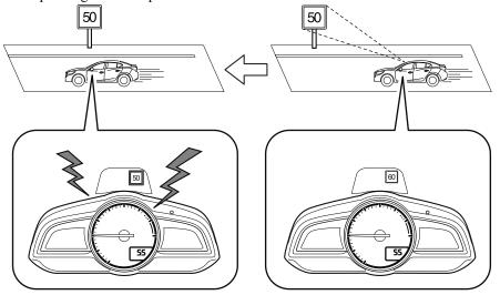
The excessive speed warning is initially set to inoperable. If you want to activate the excessive speed warning, change the setting in the personalization features. In addition, the warning pattern and the warning activation timing differ depending on the setting contents. Refer to Personalization Features on page 9-12.
