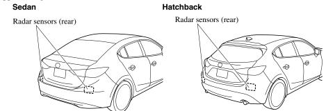
The radar sensors (rear) are installed inside the rear bumper, one each on the left and right sides.
