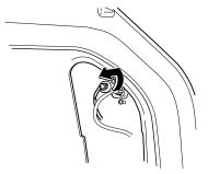
6. Disconnect the connector from the unit by pressing the tab on the connector with your finger and pulling the connector.
