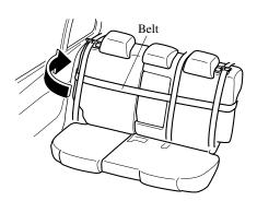
**NOTE**Pass the belt underneath the seatbelts.
