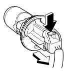
Brake lights/Taillights/Rear side-marker lights (Bulb type)
