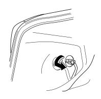
7. Disconnect the connector from the unit by pressing the tab on the connector with your finger and pulling the connector.
