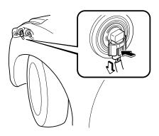
Turn the socket and bulb assembly to remove it. Carefully remove the bulb from its socket in the reflector by gently pulling it straight backward out of the socket.
