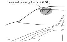
The Forward Sensing Camera (FSC) determines the conditions ahead of the vehicle while traveling at night and detects traffic lanes. The distance in which the Forward Sensing Camera (FSC) can detect objects varies depending on the surrounding conditions.
