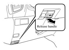
2. Insert your hand into the hood opening, slide the latch lever to the right, and lift up the hood.
