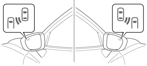
When the ignition is switched ON, the warning indicator light turns on momentarily and then turns off after a few seconds.
