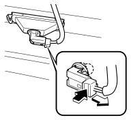
5. Turn the socket and bulb assembly counterclockwise and remove it.
