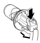
Brake lights/Taillights/Rear side-marker lights (Bulb type)
