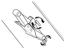
11. Turn the wing bolt completely to secure the jack.
