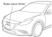
If the Smart Brake Support/Smart City Brake Support (SBS/SCBS) Warning Light (amber) is illuminated, the area around the radar sensor may be dirty. Refer to "Warning Guidance" in the center display (Type B audio).
