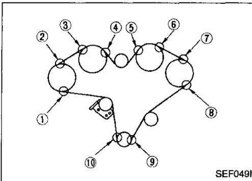
18. Check the proper installation (no slip or misplacement) of timing belt at each position as shown.
