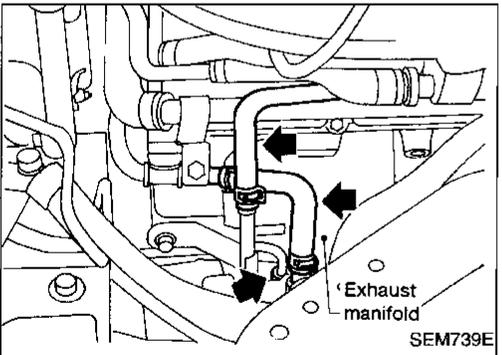
7. Remove turbocharger water hoses, and disconnect turbocharger oil inlet tube.
