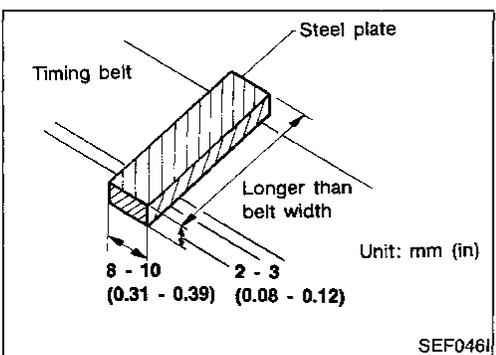
14. Prepare a suitable steel plate to measure belt deflection as shown.
