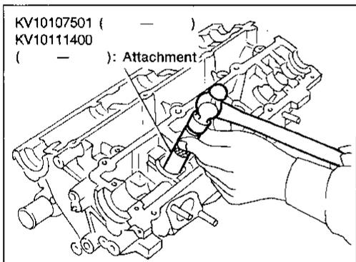
6. Apply engine oil to new valve oil seal and install it.
