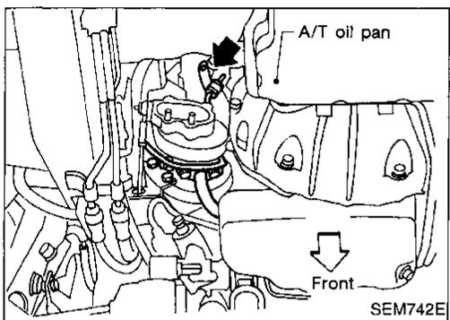
9. Remove turbocharger oil return tube and water tubes.
