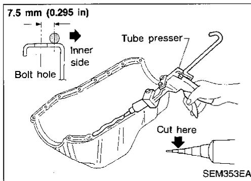
3. Apply a continuous bead of liquid gasket to oil pan mating surface.
