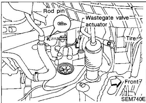
11. Remove rod pin of wastegate valve actuator.
