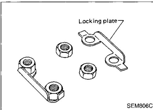
13. Unbend locking plates for fastening nuts of turbocharger unit.
