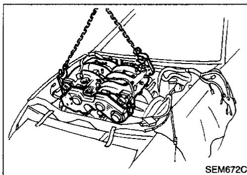
4. Remove engine from vehicle as shown.
