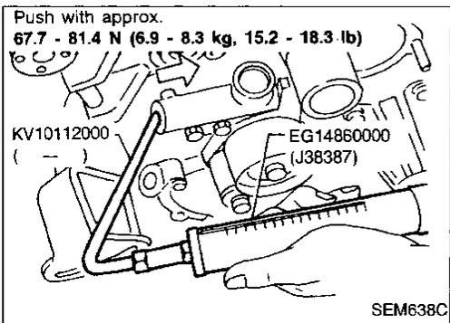
11. Push the end of pusher with approx. 58.8 N (6.0 kg, 13.2 lb) force using Tool (push-pull gauge) and tighten nut (①) and bolts (②, ③) to 16 to 21 N·m (1.6 to 2.1 kg·m, 12 to 15 ft·lb).
