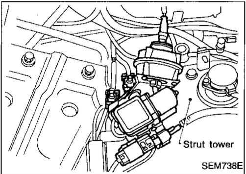
5. Remove ASCD bracket with wiper motor and solenoid valves.
