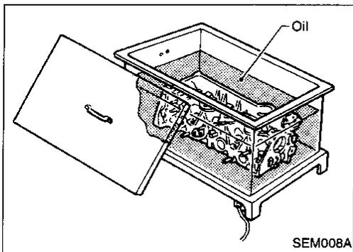
3. Heat cylinder head to 150 to 160°C (302 to 320°F).
