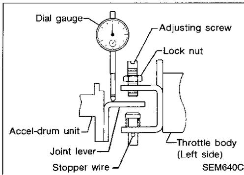
4. Set dial gauge on joint lever and set indicator to zero. Confirm that bottom end of adjusting screw is not in contact with joint lever of accelerator drum unit.
