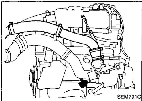
3. Remove air inlet hose and pipe.
