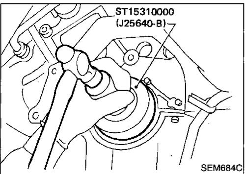
3. Apply engine oil to new oil seal and install it using Tool or a suitable tool.
