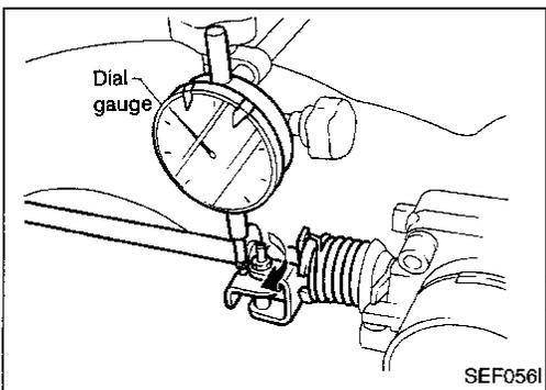
6. Turn adjusting screw until dial gauge indicates within the following range.
