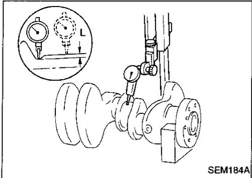
7. If clearance cannot be adjusted within the standard of any bearing, grind crankshaft journal and use undersized bearing.
