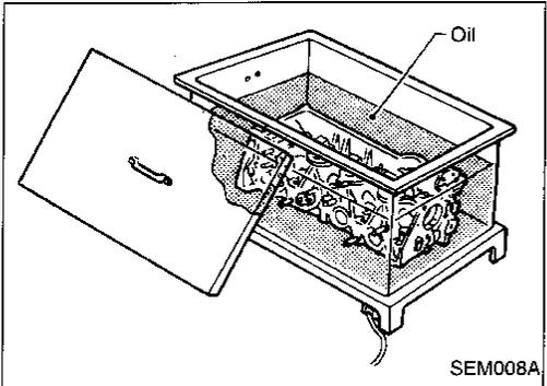
1. To remove valve guide, heat cylinder head to 150 to 160°C (302 to 320°F).
