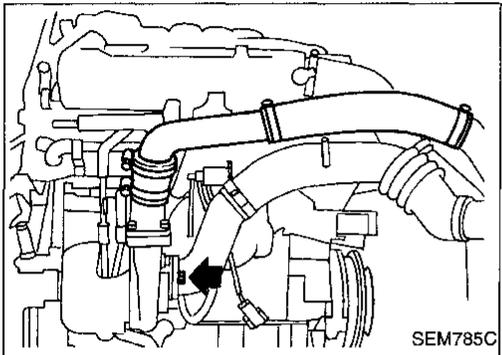
3. Remove air inlet hose and pipe.
