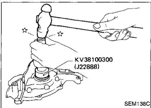
4. Apply engine oil to new oil seal and install it using Tool or a suitable tool.
