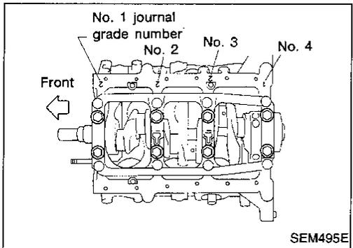
8. If crankshaft, cylinder block or main bearing is reused again, measure main bearing clearance.
