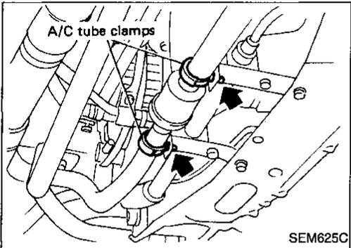
5. Disconnect A/C tube clamps as shown.
