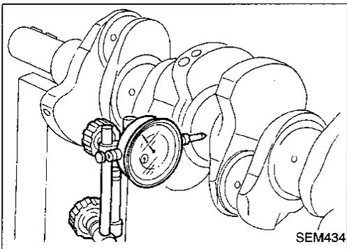
3. Measure crankshaft runout.
