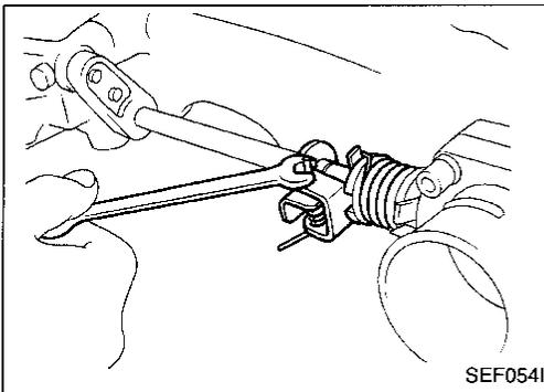
3. Loosen left side throttle body lock nut and back adjusting screw until clearance is made between the screw and joint lever.
