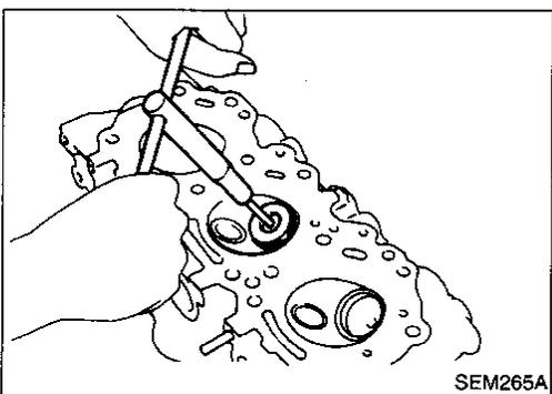
5. Cut or grind valve seat using suitable tool at the specified dimensions as shown in SDS (EM-56).
