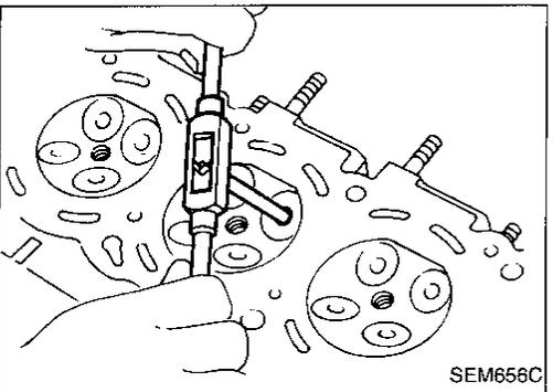
3. Ream cylinder head valve guide hole.
