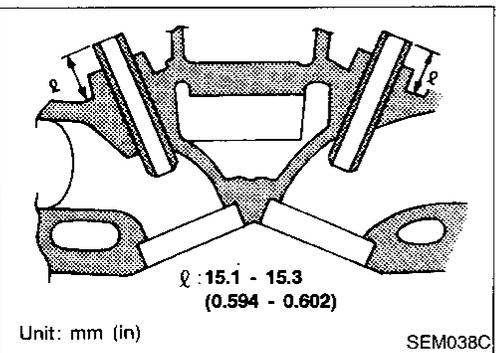
4. Heat cylinder head to 150 to 160°C (302 to 320°F) and press service valve guide onto cylinder head.
