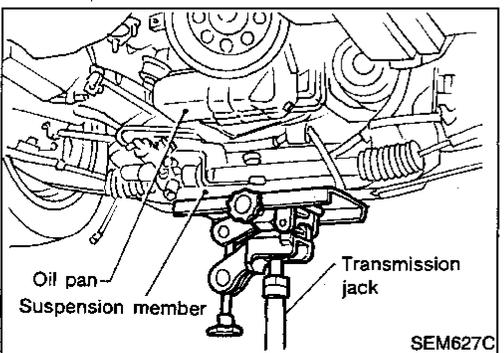
9. Set a suitable transmission jack under the suspension member.
