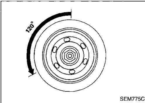
8. Turn crankshaft 120 degrees counterclockwise.
