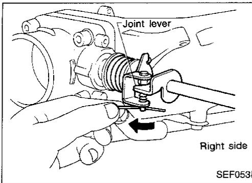
2. Pull out stopper wire of right side throttle body in order to secure right side joint lever.
