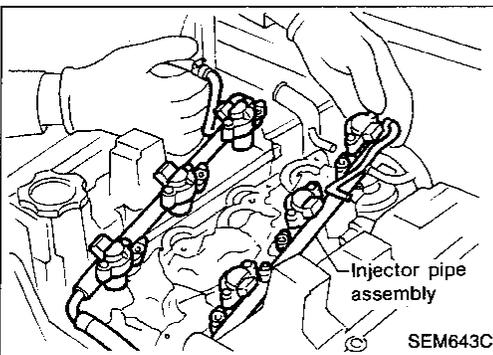
2. Remove injector pipe assembly.
