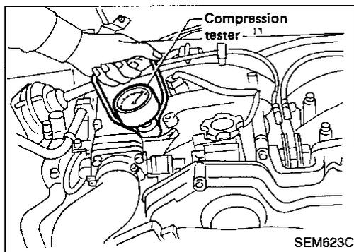
6. Attach a compression tester to No. 1 cylinder.
