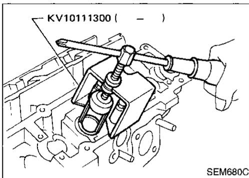
4. Remove valve spring using Tool or a suitable tool.
