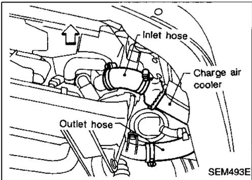
5. Remove inlet and outlet hoses.
