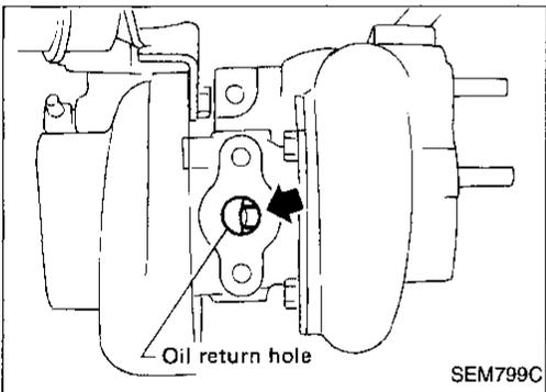
2. Check rotor shaft for carbon deposits.
