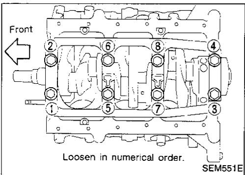
8. Remove bearing cap and crankshaft.
