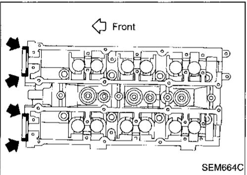
**When installing front side camshaft brackets, apply liquid gasket as shown.**
