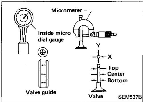
2. If it exceeds the limit, check valve stem to valve guide clearance.
