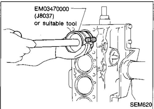
5. Install pistons with connecting rods.
