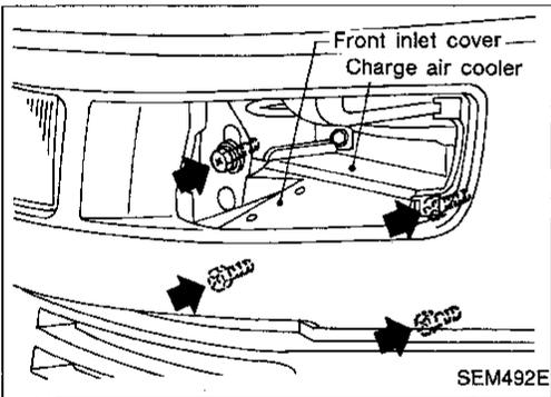
4. Remove bolts fastening charge air cooler and front inlet cover.
