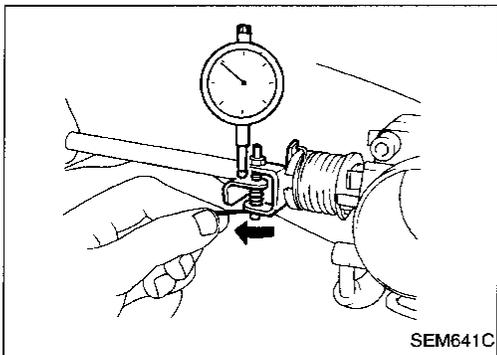
5. Pull out left side throttle body stopper wire from rod pin.
