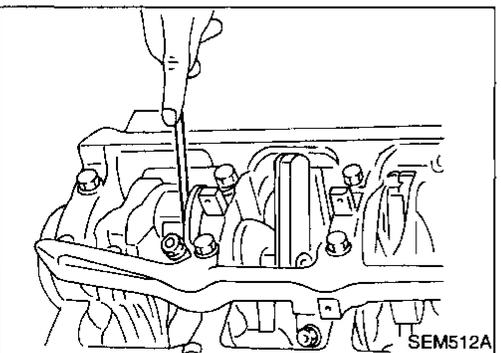
6. Measure connecting rod side clearance.
