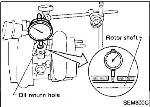
3. Measure runout of rotor shaft.
