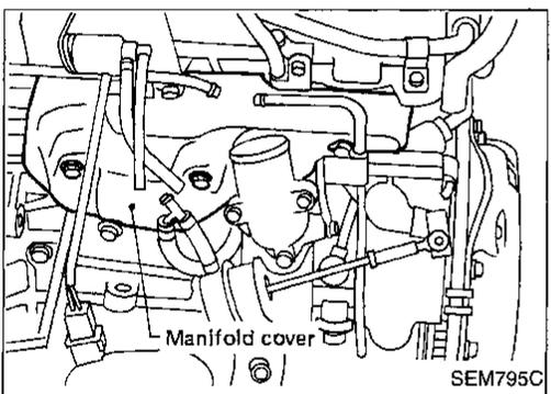
11. Remove manifold cover and fastening nuts.
