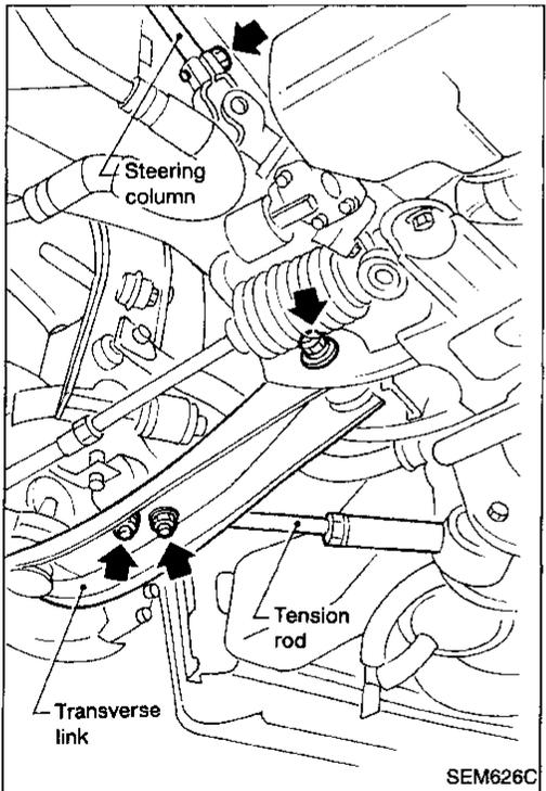
6. Disconnect steering column lower joint.
