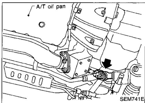
7. Remove front exhaust tube and warm up three-way catalyst.
