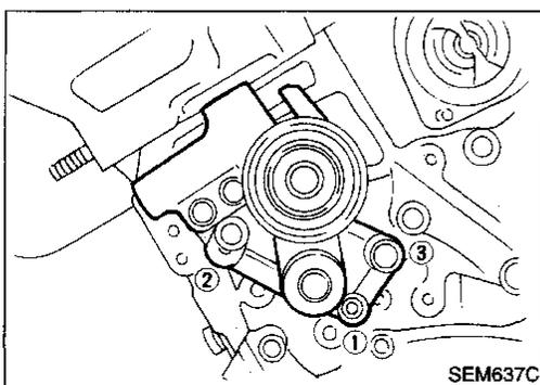
6. Install auto-tensioner and tighten nut (1) and bolts (2, 3) slightly by hand.
