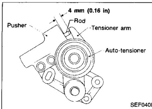
5. Using a suitable vise, adjust tensioner arm to give 4 mm (0.16 in) clearance with pusher of auto-tensioner. Then, insert stopper bolt into tensioner arm so that clearance does not change.
